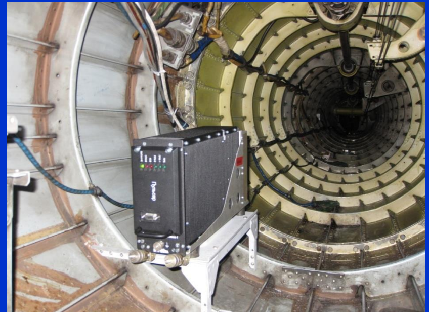
Location of Pulsar radio on board of Mi-8T RA-24105 and RA-24125 helicopters (looking aft).
