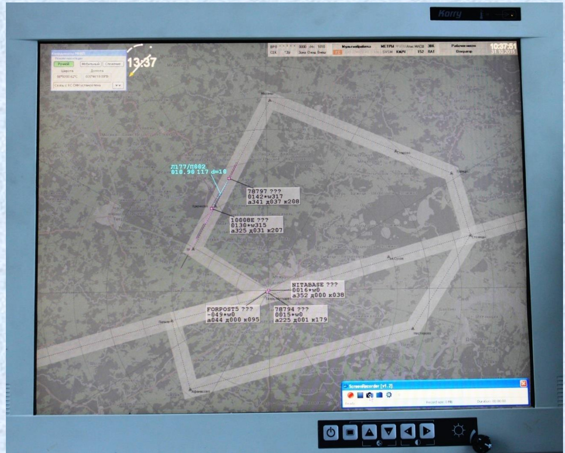
ADS-B display at the mobile command and control station
